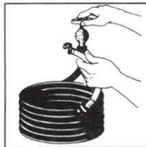
5. Holding water level tube above level of faucet, turn on water, allowing it to run freely and evenly until all air bubbles are out of hose and tube.
