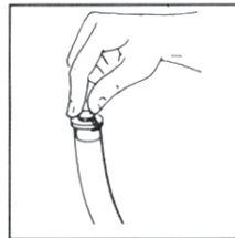
6. When all air bubbles have been cleared from tube, turn down water force slowly until completely off, and close breather cap.
